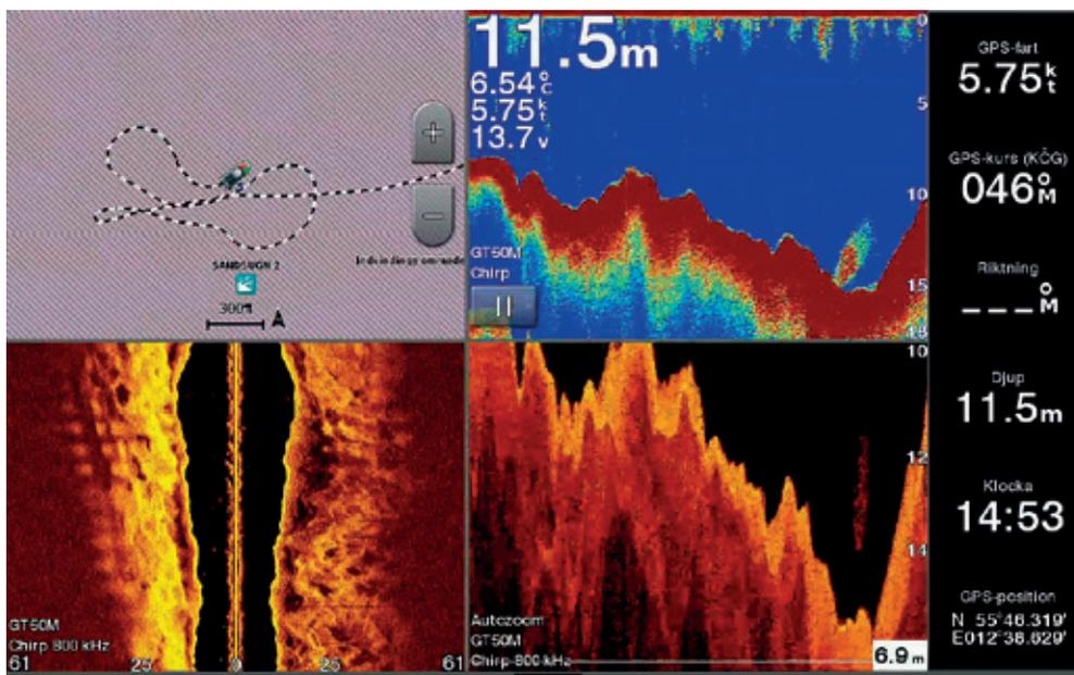
Image from the *Elias* depth sounder in a dredged area. The display in the lower right quadrant clearly shows the abrupt increase in depth at the edge of a dredging hole. © SEA-U Marint Kunskapscenter
