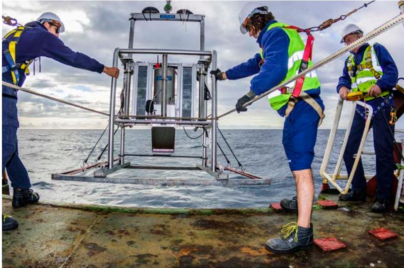
tics of the seafloor. Backscatter data were obtained using a Reson Seabat 7125 SV multibeam echosounder (Teledyne Marine), which was operated at a frequency of 200 kHz, with a maximum ping rate of 50 Hz, 256 equidistant beams, maximum swath angle
