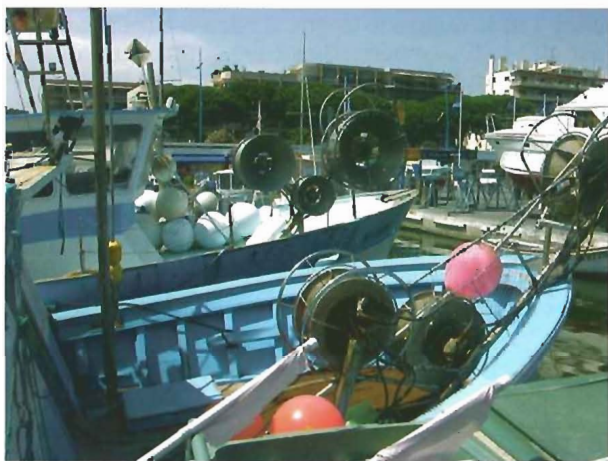
© OCEANA/Xavier Pastor. Triple-wheel net haulers belonging to two "thonaillers". La Napoule.
