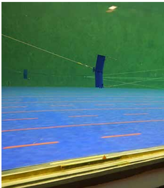
Figure 11. Semi-pelagic trawl doors tested in a water tank (Extracted from Bastardie et al. 2022).
