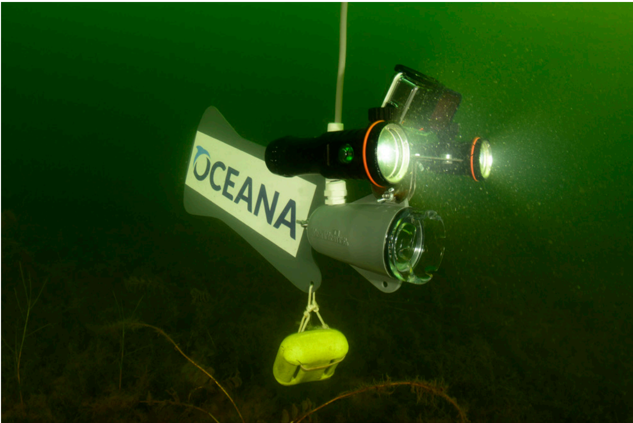
Figure 11. The drop video camera system used in the Quark 2018 surveys. The system consisted of a GoPro Hero 5 Black video camera with underwater housing, mounted on the Sea Viewer 6000 HD Sea-Drop, with two external diving torches mounted on the sides for additional lighting. The Sea Viewer system is the HD PRO PACKAGE console with live feed at the surface and recording capability ( https://www.seaviewer.com/ ). Each drop video survey point was recorded with both the GoPro (primary camera) and the Sea Viewer (secondary, back-up camera). © OCEANA/ Carlos Minguell.
